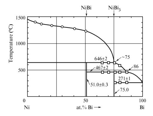
**Fig.1.15.** Equilibrium phase diagram of the Ni–Bi binary system according to the work of P. Feschotte and J.-M. Rosset.<sup>148</sup>
